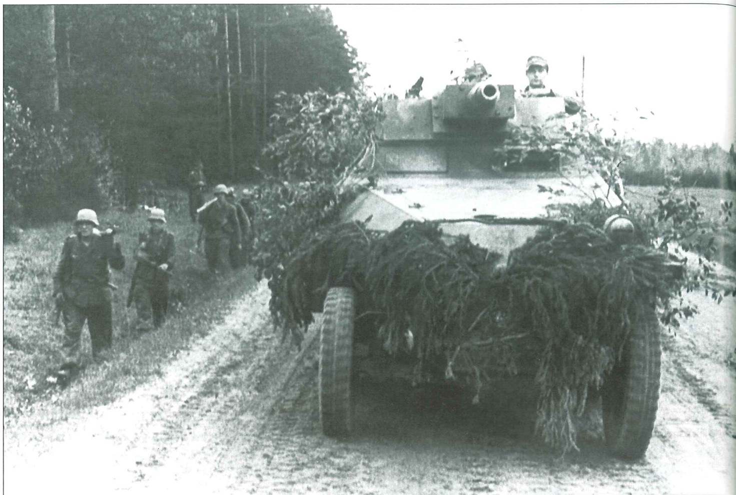
A front view of another late production "Stummel" which was produced only on the simplified Ausf.D chassis. The first version had the gun installed in the front of the superstructure to the right of the driver. This required additional work to produce, and so in 1944, when German military industry had reached its peak, it was changed to make construction simpler. This "251/9" belonged to the Panzer-Grenadier-Division "Großdeutschland" during the battles around Memel in the fall of 1944. Note the coaxial MG42 on the left.
