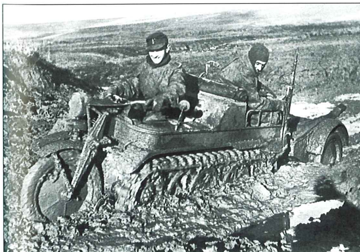
Though completely covered in mud, this Kettenkrad is still immediately recognizable. The Kettenkrad was the perfect vehicle for such terrain where it was impossible for standard motorcycles to operate. Not a light vehicle, weighing about 1,280 kg., its 36 hp engine was capable of propelling it, with its 2-3 man crew and 450 kg. capacity trailer, through the worst Russian mud, as can be seen in this photo.
