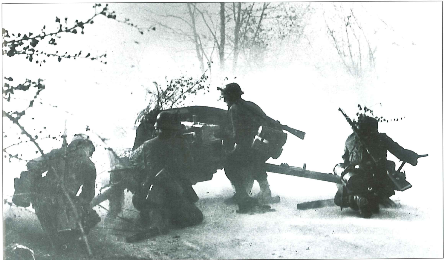
A Pak 40 in action in Italy, spring 1944. The crew appears to have had no time to prepare their position before entering into the battle, as two of them are holding the ends of the gun trails down to prevent the gun from moving when fired. Note the foliage attached to the end of the barrel completely covering the muzzle brake. The smoke of battle has almost obscured the battlefield.
