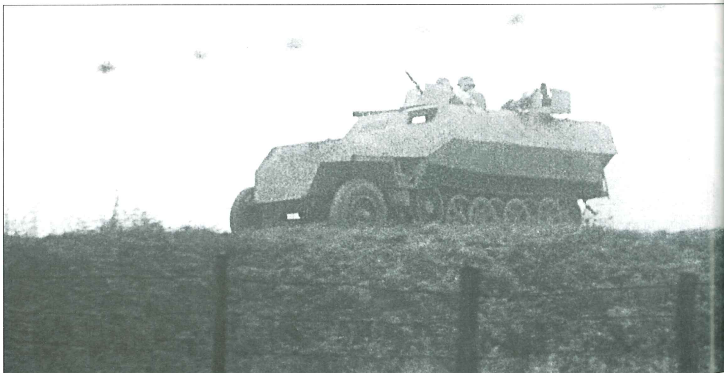
The Sd.Kfz.251/16 flame thrower model was introduced in January 1943 into the Pionier battalions of the Panzer divisions and later on in a few of the best equipped Panzergrenadier divisions. It carried two 700 liter flame fuel tanks in the rear of the compartment which allowed for approximately 80 short bursts to a range of up to 35 meters. This one is photographed somewhere in Western Europe in the late summer of 1944. The APC has no markings which was not unusual, for vehicles were often sent into combat as soon as they were received.
