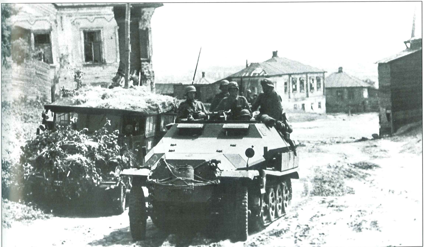
Another Sd.Kfz.251/1 Ausf.C of 24.Panzer-Division passing a Mercedes-Benz L1500A personnel carrier while travelling through a village in the Stalingrad area, early autumn of 1942. The divisional emblem and national cross are also visible on the engine deck as in the previous photo. Note the metal food container attached to the front plate with the tow cable and the lack of MG shield.
