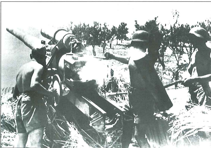
A 15cm sIG 33 howitzer camouflaged with white paint, winter 1942. It was considered a good infantry support gun, even though it was heavy by the standards of that time, and it remained in service until 1945. A number of these guns were mounted on a variety of self propelled chassis as well. It was utilized on the regimental level for direct fire support during attacks.
