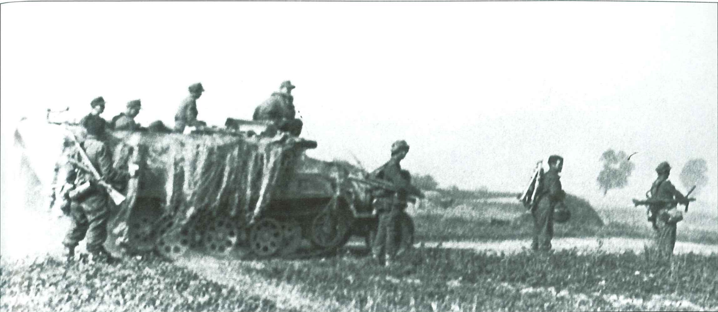
The artillery support model of the Sd.Kfz.251 is known as the "251/9". It was armed with the old, short barrel 7.5cm KwK 37 L/24 which had been previously installed in Panzer IV Ausf.A to Ausf.F1 in the spring of 1942. Here we have an example of such a vehicle, camouflaged with straw and photographed in early autumn 1944 during the battles against the Russian bridgehead on the Vistula River in Poland. In 1944, there were 23 Sd.Kfz.251s in each Panzergrenadier company with three for the headquarters section, 3 platoons with 4 vehicles each and a heavy weapons platoon with 8 vehicles. In the heavy weapons platoon there were 3 Sd.Kfz.251/17 for anti-aircraft protection, 2 Sd.Kfz.251/9 and 2 Sd.Kfz.251/2 armed with the 8cm mortar plus an Sd.Kfz.251/1 for the platoon leader.
