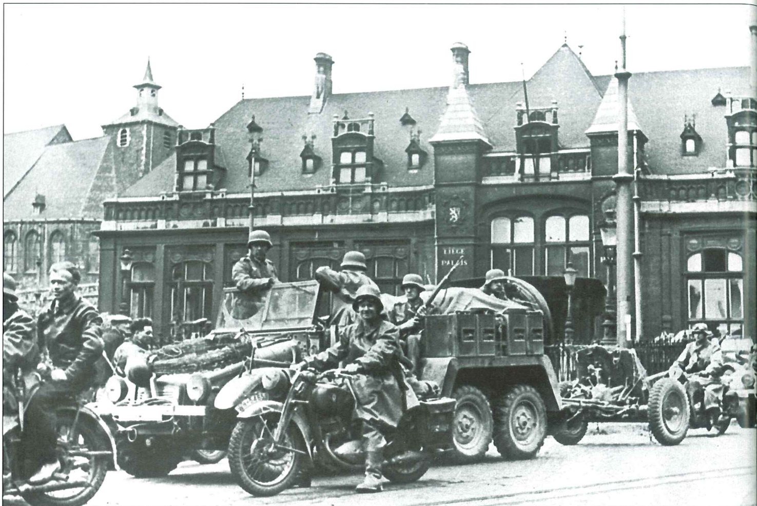
A column from a Panzerjäger Abteilung halted on a street in Liege, Belgium during the "Blitzkrieg" in May 1940. The vehicle seen behind the DKW NZ350 motorcyclist is the famous Krupp Protz Kfz.69 being used as a tractor for the 3.7cm PaK 36 anti-tank gun. This version varied from the Kfz.70 personnel carrier in the rear part only, where the seats for an infantry squad were replaced by ammunition racks and seats for the gun crew. There is a roll of barbed wire and a French helmet on the front of the vehicle. Note the civilian rider on the motorcycle on the left.
