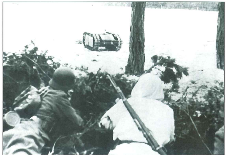
This is the first model of "Goliath" produced, the electric drive Sd.Kfz.302. Here it is being maneuvered toward an armored target - an SU-85. It carried a 60 kg. explosive charge that could cause severe damage to an armored vehicle but it was highly vulnerable to ground fire and was not as effective a weapon as the later Sd.Kfz.303. This is a propaganda photo that was taken in the winter of 1943/44.
