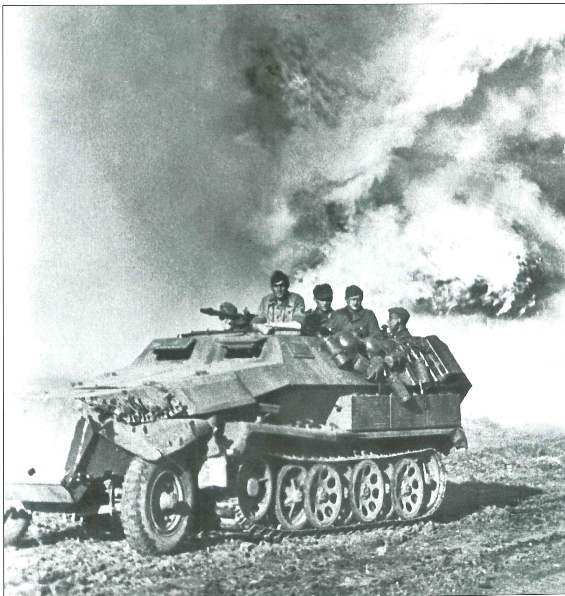
Another burning farm passed by an Sd.Kfz.251/1 Ausf.C, again, without the MG shield and missing the mudguard on the front wheel. Of special interest is the camouflage and markings on this vehicle. The chassis is covered with dust and mud of course, but the rest of the vehicle has a dark green camouflage sprayed over the dark gray base. The tactical number is in yellow and is in the standard 3 digit configuration indicating the 3rd vehicle in the 2nd platoon of the 5th company. The rod antenna for the Fu.Spr.Ger. F radio was most commonly located as shown but was often located in the middle of, or rear end of, the side plate and sometimes tilted at an angle toward the inside of the vehicle.
