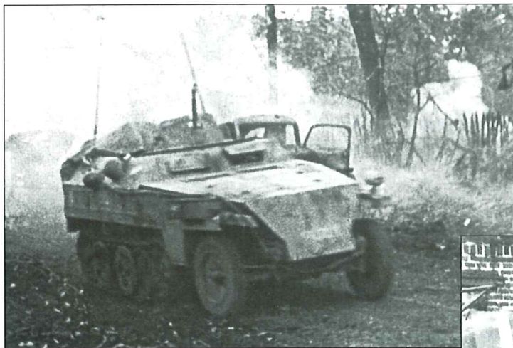
A lone Sd.Kfz.250/1 "Neu" of a Wehrmacht unit passes through the debris of a demolished caravan of German refugees somewhere in the Polish-Lithuanian-German border area in the autumn of 1944. The "Neu" version of the Sd.Kfz.250 was the same basic vehicle as the "Alte" version but with much simplified construction that makes it look like a completely different vehicle. The mudguard over the tracked part of the chassis was integrated with a stowage compartment and the fighting compartment and engine deck were widened.
