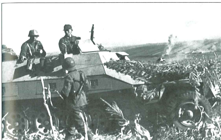
The Pionier version of the Sd.Kfz.251 was probably one of the rarer APCs. Here we see one of them from an unknown division during the battles around Zhitomir in the autumn of 1943. There is a unit emblem visible on the upper right corner of the front plate very similar to that of s.Pz.Abt.507. The Sd.Kfz.251/7 were assigned to the 3rd company in each Pionier battalion. The light assault bridges carried on the sides of the vehicle were very useful for crossing ditches or narrow streams during attacks.
