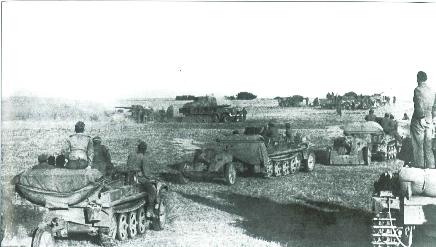
A Panzerjäger Abteilung equipped with Sd.Kfz. 10s and towed 5cm PaK 38s, the barrels of which have been removed by the censor, passing a battery of 8.8cm FlaK 36 guns at work in the Stalingrad area in September 1942. The PaK 38 was still the main anti-tank weapon in the Panzerwaffe at this time as the more powerful 7.5cm PaK 40 had been only in service a few months. The situation was similar with transport - the Sd.Kfz. 10 was the most common prime mover in these units as well, mainly due to the high speed and cross country capabilities of this half-track. Seen at the right is a Pz.Kpfw. III Ausf. J.
