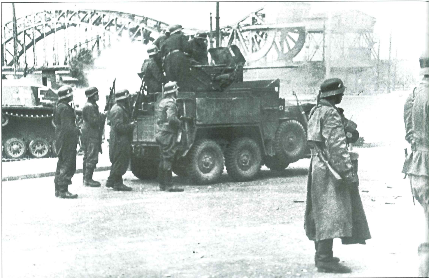
A Krupp Protz fitted with a 2cm FlaK 38 supporting a Sturmgeschütz Abteilung in a Lithuanian city during the summer of 1941. It was a very rare modification of the Protz. The FlaK 38 was mounted on special supports installed in the standard body of the Kfz.81, usually utilized for the gun crew and ammunition. The first such anti-aircraft vehicles were put into service in 1941 along with similarly modified Horch cross-country cars. The StuG.III Ausf.B or C in the background has an unusual marking painted on the side in front of the national cross. The Luftwaffe troops in the picture are wearing the standard Fliegerbluse, which was cut shorter than the standard army tunic, and the one piece dark blue-gray or black twill fatigue uniform. The soldier second to right is wearing a motorcyclist's waterproof coat.
