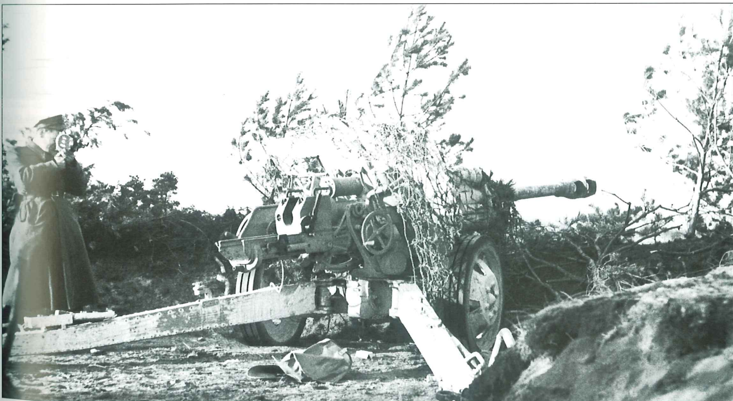
The Germans very often used captured Soviet guns. This one is a 76.2mm Model 1939 division gun, developed and used as a dual purpose gun by the Soviets and designated 7.62cm FK 297(r) or 7.62cm PaK 39(r) in German service. It was used by the Germans the same way as the Soviets used it even though it was not as effective as the 7.5cm PaK 40. The high shield made this gun more difficult to conceal and provided less protection from machine gun bullets and shell splinters for the crew. The gun was repainted with overall sand and has a worn white winter camouflage paint coat.
