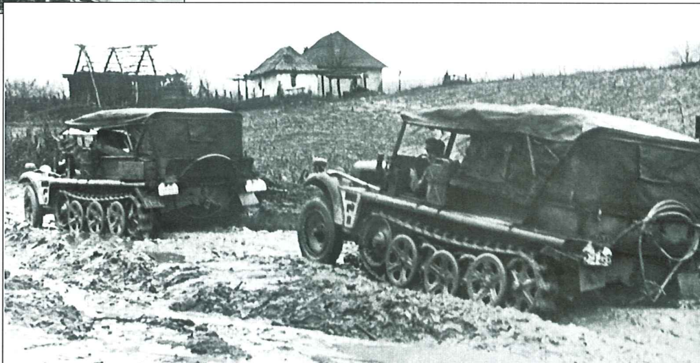
The standard transport version of the Sd.Kfz. 10 following the anti-aircraft version of the same type of half-track, either an Sd.Kfz. 10/4 or 10/5, Volchov area, September 1942. During wet weather, half-tracks, especially the light ones, were the best form of transportation and so were very often employed by various staffs in the divisions.
