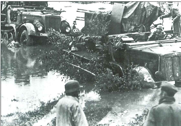
The anti-aircraft Sd.Kfz. 7/2 consisting of the medium prime mover and the 3.7cm Flak 36 anti-aircraft gun. The vehicle was less common than the Sd.Kfz. 10/4 (ratio 1:3) and this version was rather very rare up to the end of 1942. Here we see one of these vehicles from an independent Luftwaffe AA battalion on harbor defense in Southern France in November 1942. The crew members have tropical uniforms and the half-track is painted in overall sand. Note the boxes of ammunition and crew equipment fixed to the lowered sides.
