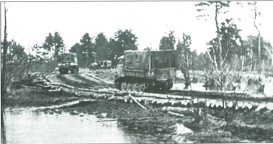
An anti-tank team from an SS division travelling through the western Soviet Union riding on a 7.5cm PaK 97/38(f) anti-tank gun towed by an RSO/01 fully tracked tractor. Both the vehicle and the gun are painted with overall sand without any camouflage pattern, which usually indicated they were rushed to the front from the factory and placed into service immediately. Note that four of the gun crew are wearing the first type of SS winter uniform, the fur lined anorak, a pullover which featured an oversize hood designed to be worn over the helmet. The weather must be mild as the soldier sitting on the left is playing an accordion.
