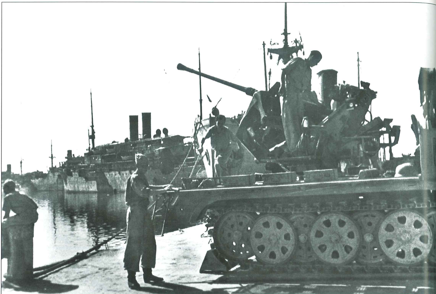
The anti-aircraft Sd.Kfz. 7/2 consisting of the medium prime mover and the 3.7cm Flak 36 anti-aircraft gun. The vehicle was less common than the Sd.Kfz. 10/4 (ratio 1:3) and this version was rather very rare up to the end of 1942. Here we see one of these vehicles from an independent Luftwaffe AA battalion on harbor defense in Southern France in November 1942. The crew members have tropical uniforms and the half-track is painted in overall sand. Note the boxes of ammunition and crew equipment fixed to the lowered sides.
