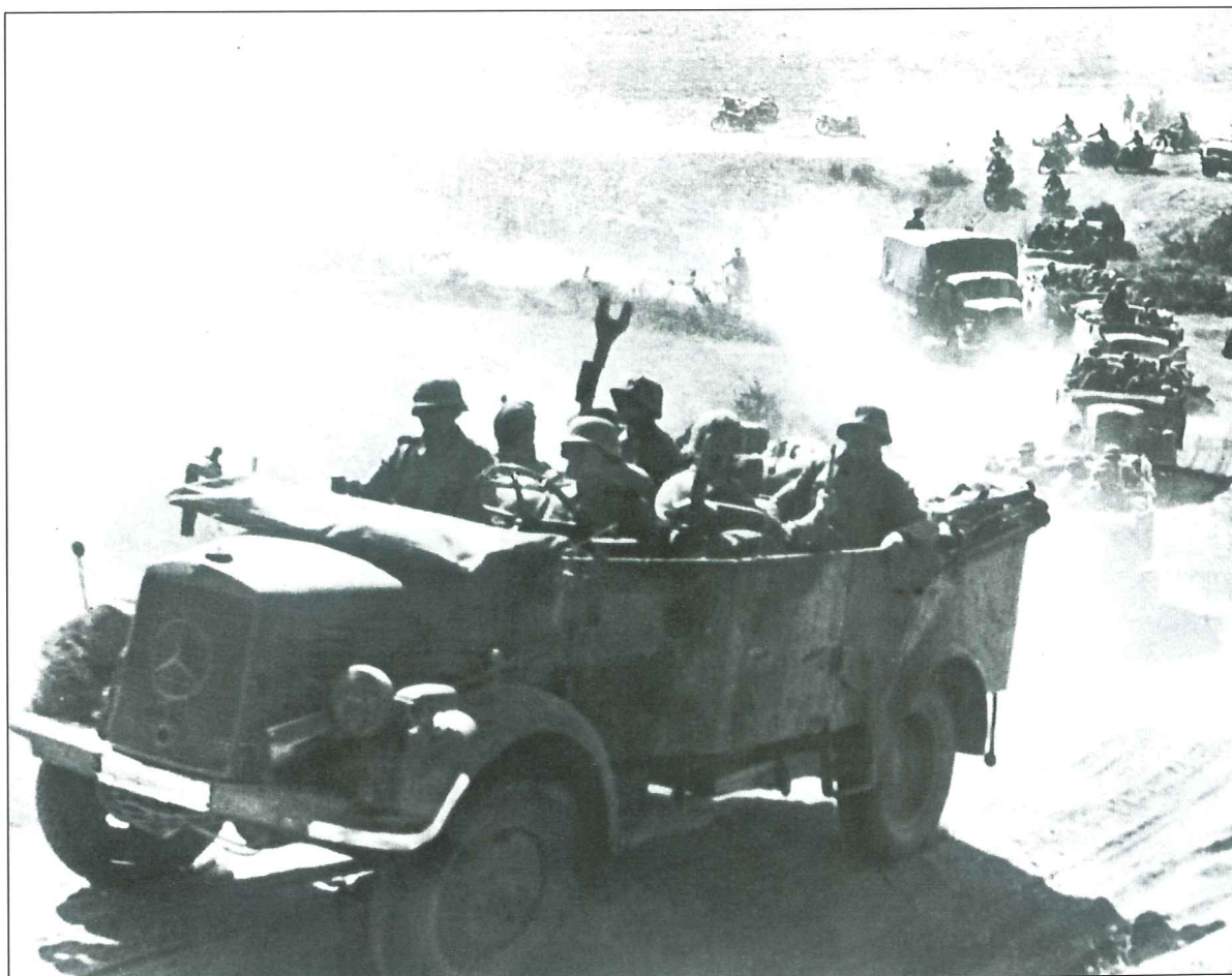
A column of cars and trucks during a march break, probably somewhere in Western Germany during the early stages of the war. The column is guarded by a 2cm FlaK 30 light anti-aircraft gun while other similar weapons are being towed by the Krupp Protz Kfz.69 in the background. This was the most common type of towing vehicle during this period and was replaced by the heavier Horch 1a later on. Note the details of the 2cm gun and sight in the foreground.
