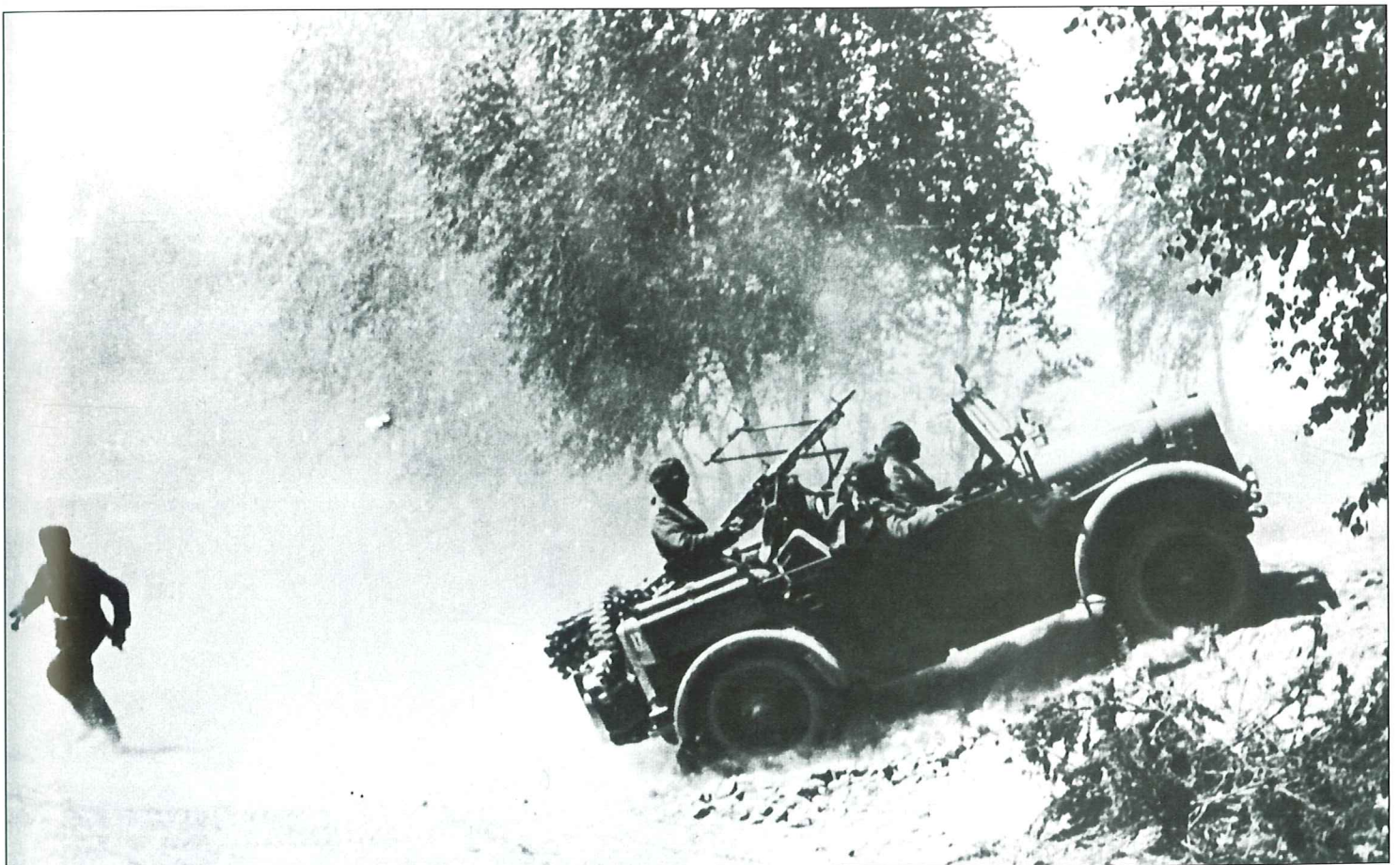
The Kfz.4 was classified as a light cross-country car but was more rugged than the Kfz.12. It was produced on the chassis of the Ein.Fahr.1 für le.Pkw (standard chassis 1 for light army car) by BMW, Hanomag and Stoewer and is seen here driving off the road to engage an enemy target. The dual MG34 installation seen on the back of this Stoewer 40 was a typical light anti-aircraft mount widely used in all Wehrmacht divisions during the early stages of the war and was installed on other types of light cross-country cars as well.
