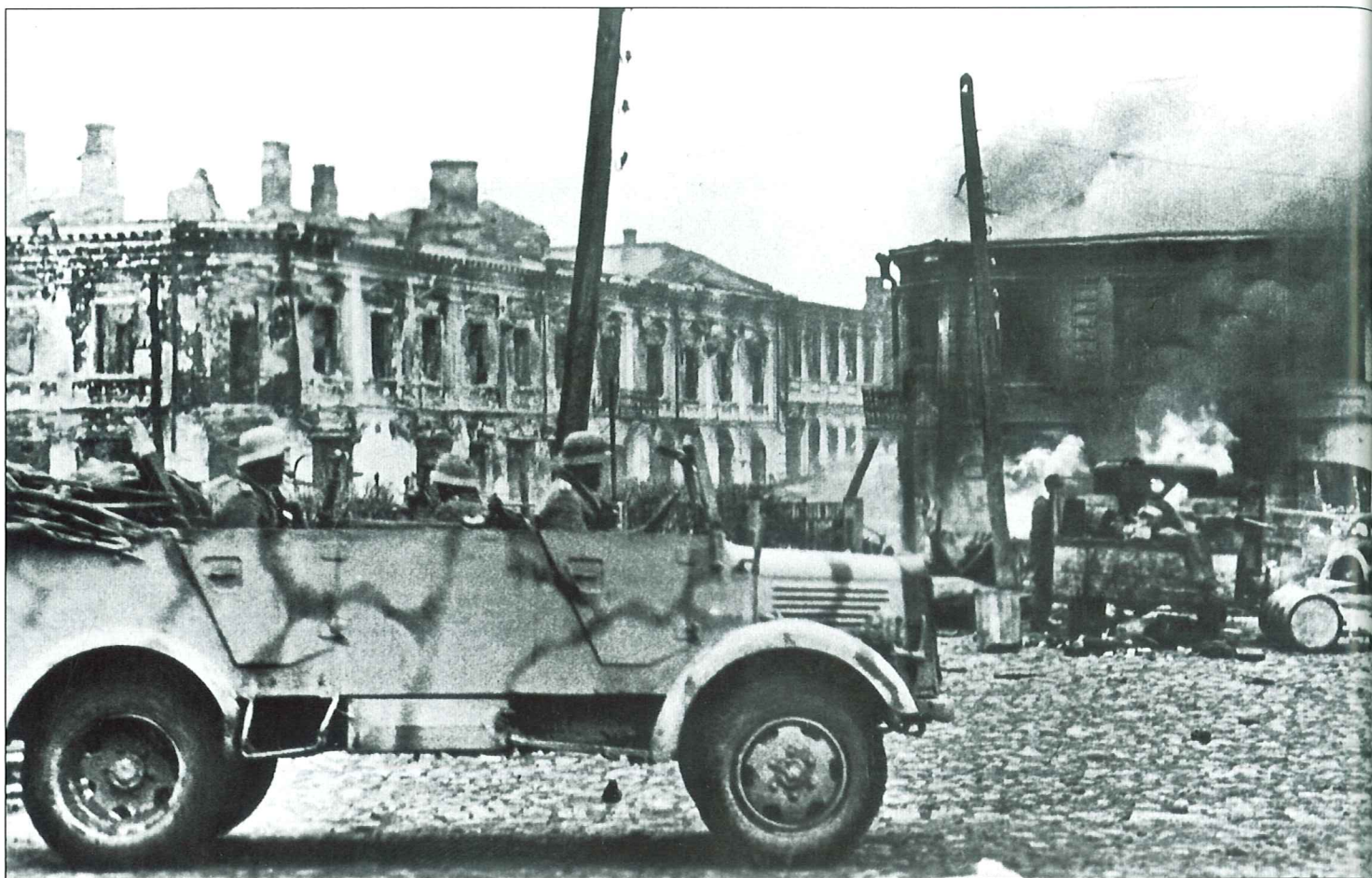
Another Mercedes-Benz Type L 1500A. The s.gl.Pkw (schwere geländegängiger personenkraftwagen) Kfz.21, also produced by Steyr and Phänomen-Granit, served as infantry transport vehicles and as le.gl.Lkw (leichter geländegängiger lastkraftwagen) Kfz.69 light anti-tank gun tractors and Kfz.81 light anti-aircraft gun tractors. The vehicle is painted in overall sand yellow and camouflaged with a wavy brown pattern, typical for autumn. It is driving through Zhitomir in December 1943 after the recapture of the city by 7.Panzer-Division, the last spectacular offensive victory of the Wehrmacht in the Soviet Union.
