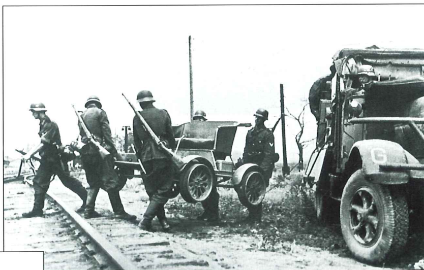
A railroad trolley is unloaded from a Henschel 33 G 1 diesel engined medium truck from one of the Panzer divisions of Panzergruppe Guderian in the Soviet Union during the summer of 1941. This type of equipment was very useful in Russia due to their vast railway network and lack of good quality roads.
