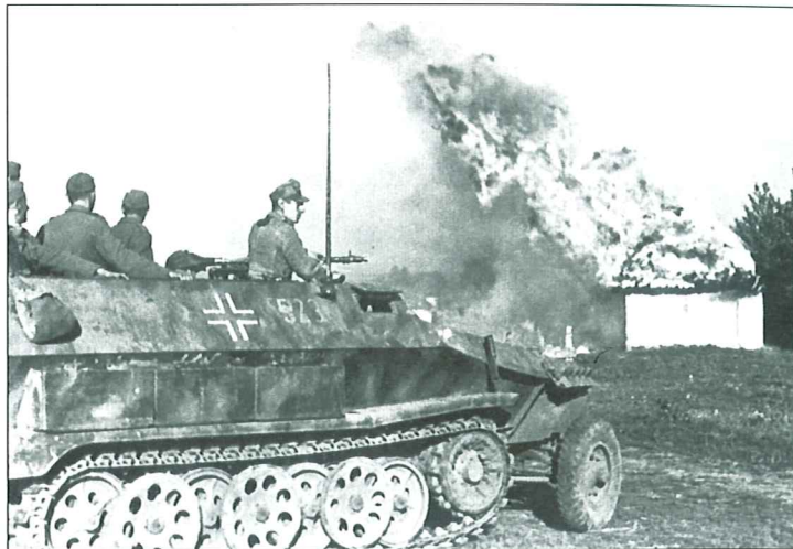
Another burning farm passed by an Sd.Kfz.251/1 Ausf.C, again, without the MG shield and missing the mudguard on the front wheel. Of special interest is the camouflage and markings on this vehicle. The chassis is covered with dust and mud of course, but the rest of the vehicle has a dark green camouflage sprayed over the dark gray base. The tactical number is in yellow and is in the standard 3 digit configuration indicating the 3rd vehicle in the 2nd platoon of the 5th company. The rod antenna for the Fu.Spr.Ger. F radio was most commonly located as shown but was often located in the middle of, or rear end of, the side plate and sometimes tilted at an angle toward the inside of the vehicle.
