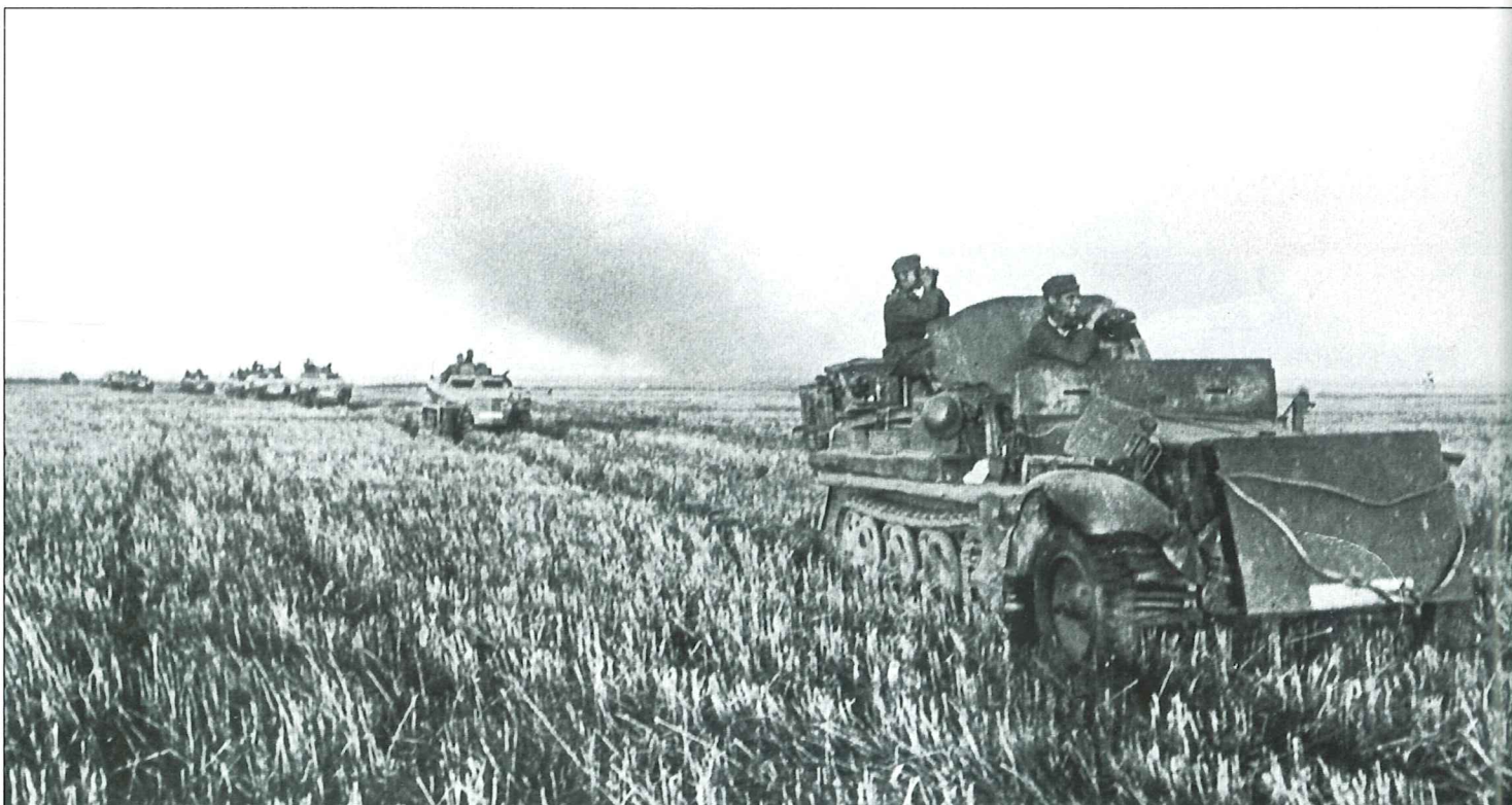
A 5cm PaK 38(sf) auf zugkraftwagen 1 t with armored shields for the engine and driver is leading a column of Sd.Kfz.250 across a field in the Kuban, August 1942. The Sd.Kfz.10 was used mainly as the carriage for the 2cm FlaK 36 anti-aircraft guns in the 10/4 and 10/5 versions, but in 1941 a small number of the Demag D7 were fitted with the 3.7cm Pak 36 anti-tank gun by their crews after their combat experiences of the previous year. Later on, often in field workshops, armored plates were installed on many of them and the armament increased. Here, the censor has removed the long L/60 barrel of the 5cm PaK 38 anti-tank gun.
