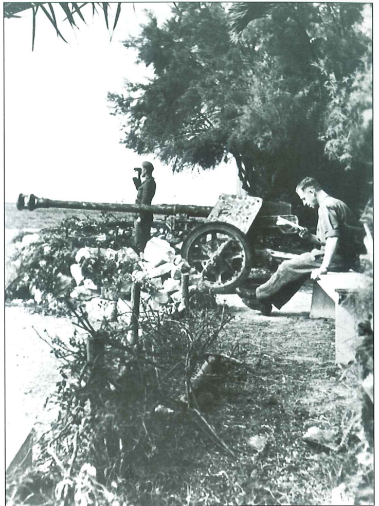
A profile shot of a 7.5cm PaK 40 in the Soviet Union in 1942. The bolt heads on the outside of the gunshield had holes, through which wire could be strung to attach foliage as camouflage. The gun could be fired with the foliage attached and even moved to a new position if needed. If there was any wind on the battlefield, it was difficult to spot these camouflaged guns as the wind dissipated the smoke.
