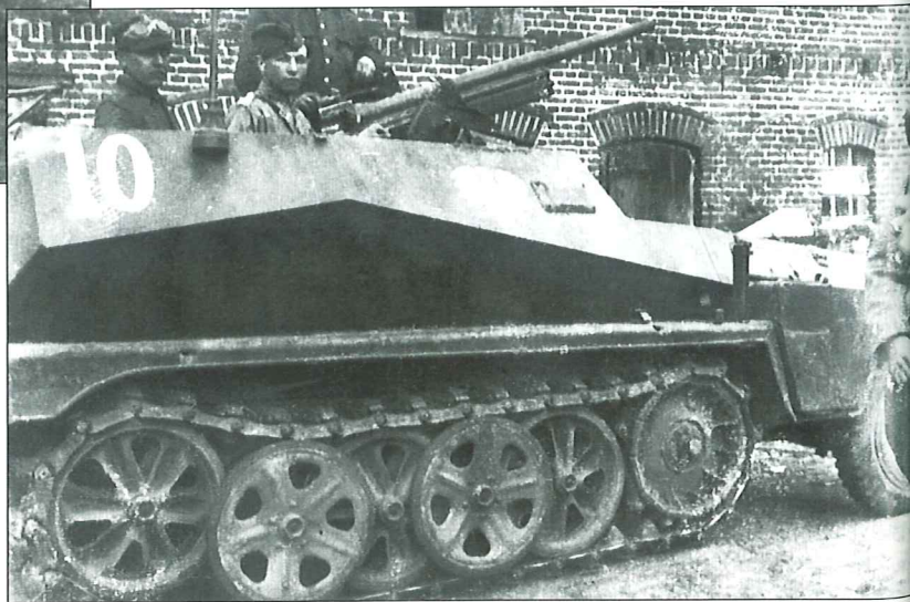
An Sd.Kfz.250/3 "Neu" radio communications vehicle races through a village near Goudap in Pomerania to avoid Soviet artillery fire. The 250/3 model was built in several versions and employed by different command levels for radio liaison duties linking them with the Luftwaffe and heavy artillery units. The main difference from the standard 250/1 model was the installation of FuG 7, FuG 8 or FuG 12 radios, which could be recognized by the long rod antenna installed on the left rear of the combat compartment. Here we have a vehicle with one of these antenna, while the one on the right side is for the standard Fu.Spr.Ger. F radio set carried by each vehicle.
