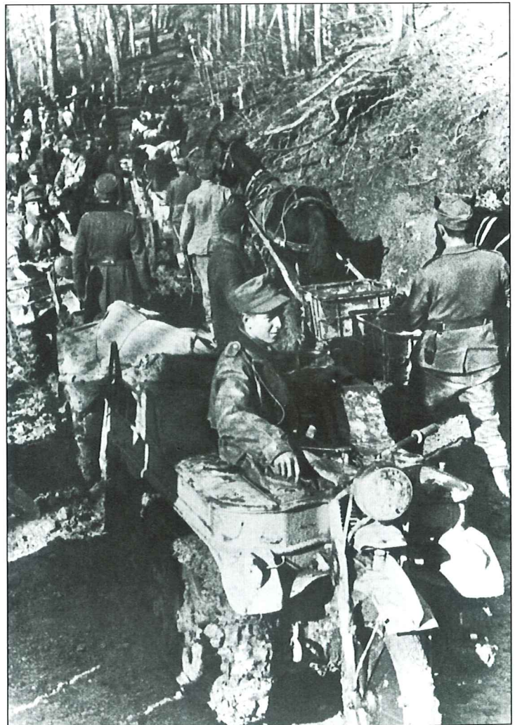
Here we see a group of three Kettenkrads waiting for a column of horse drawn carts to pass by on a narrow path over hilly terrain. All of them are loaded down with equipment which also completely fills the trailer attached to the leading Sd.Kfz.2. It can be seen that these vehicles have been through some difficult, muddy conditions as well.
