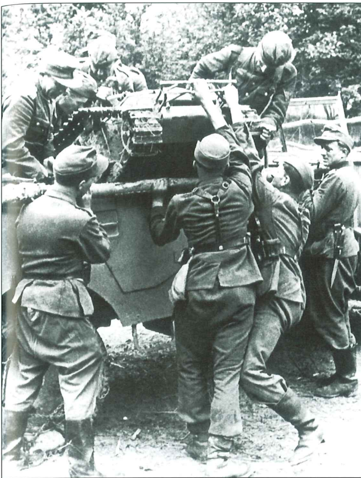
This is the first model of "Goliath" produced, the electric drive Sd.Kfz.302. Here it is being maneuvered toward an armored target - an SU-85. It carried a 60 kg. explosive charge that could cause severe damage to an armored vehicle but it was highly vulnerable to ground fire and was not as effective a weapon as the later Sd.Kfz.303. This is a propaganda photo that was taken in the winter of 1943/44.
