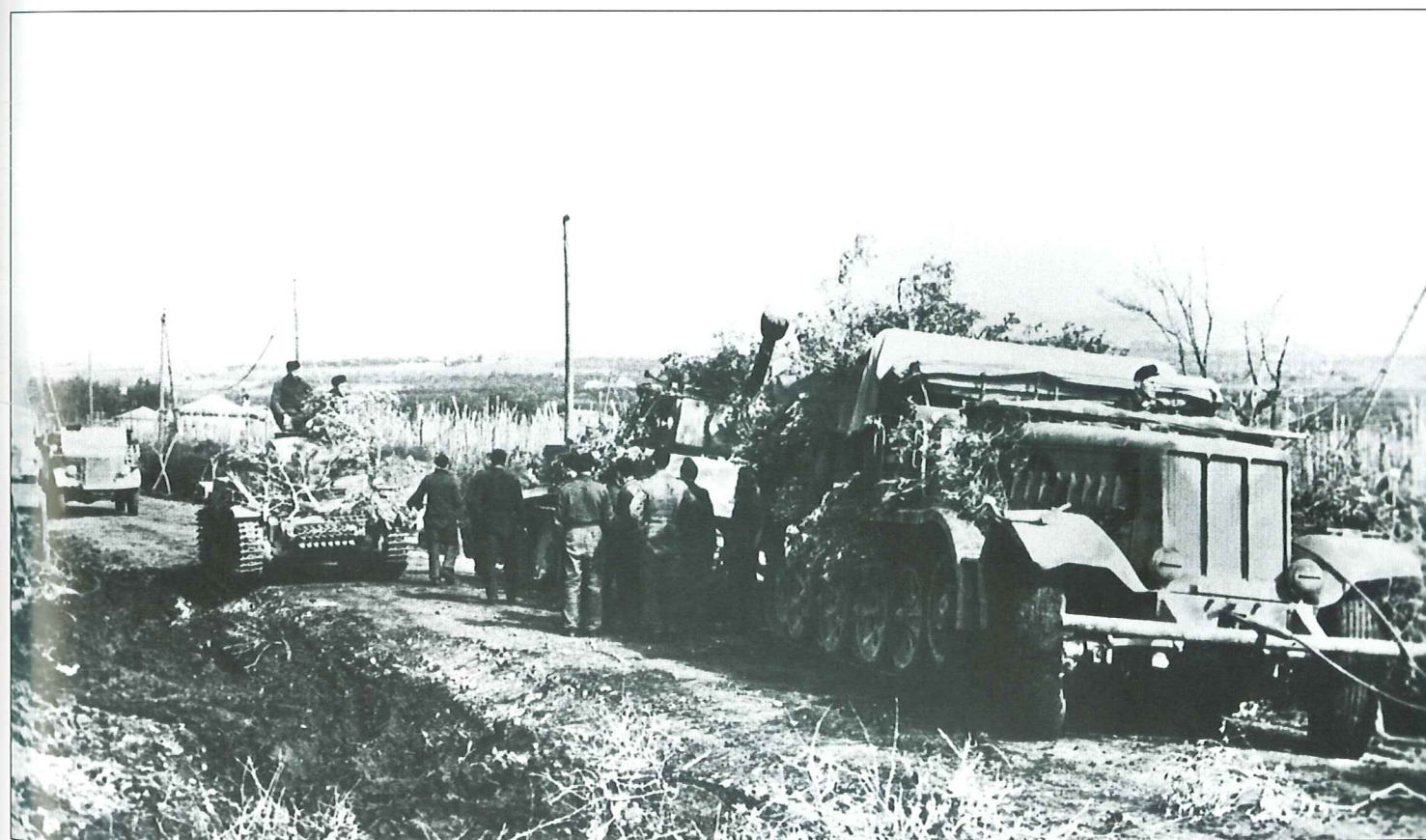
An Sd.Kfz.7/1 camouflaged with foliage and painted with a wavy green pattern on an overall sand base passing burning houses in a city recaptured from Soviet hands somewhere on the Polish-Russian border, summer 1944. The same pattern has been applied on the trailer as well as the half-track, which bears a "WH" prefix license plate. This vehicle is unusual in that it is only partially armored.
