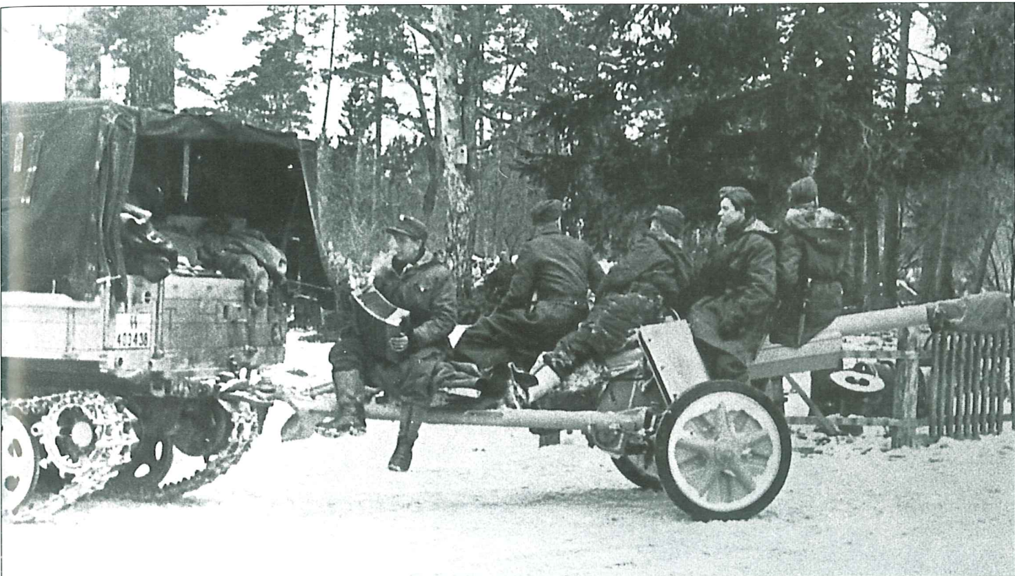
An anti-tank team from an SS division travelling through the western Soviet Union riding on a 7.5cm PaK 97/38(f) anti-tank gun towed by an RSO/01 fully tracked tractor. Both the vehicle and the gun are painted with overall sand without any camouflage pattern, which usually indicated they were rushed to the front from the factory and placed into service immediately. Note that four of the gun crew are wearing the first type of SS winter uniform, the fur lined anorak, a pullover which featured an oversize hood designed to be worn over the helmet. The weather must be mild as the soldier sitting on the left is playing an accordion.
