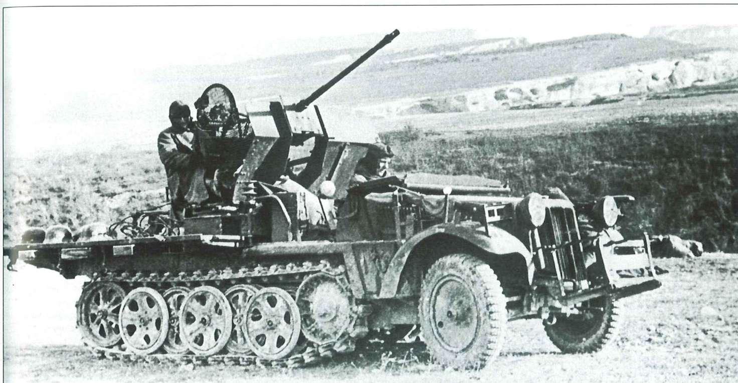
A frozen crew of a self propelled anti-aircraft gun waiting for the enemy to appear somewhere in the Crimean Peninsula, December 1942. The first Demag D7 with 2cm FlaK 30 were introduced into frontline units in early 1939, and so saw service in Poland in September that year. The vehicle had a totally different rear compartment than the standard version of the Sd.Kfz.10, as the seating for the 8 men squad was replaced by a platform for the gun. In this configuration, the vehicle was designated Sd.Kfz.10/4 and when the armored cab was added, Sd.Kfz.10/5. Produced in large numbers, it was the most common anti-aircraft vehicle in the Wehrmacht during WWII.
