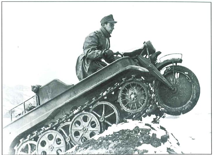
The NSU HK100 (Sd.Kfz.2), known as the kleines Kettenkraftrad, or Kettenkrad for short, was a completely different kind of motorcycle. Small and quite fast, with a maximum road speed of 70 kmh (cross country 50 kmh), it could travel across difficult terrain, crossing narrow forest tracks and desert expanses equally well. This photo shows very well the tracked chassis of the Kettenkrad which was constructed similar to the Sd.Kfz.10, Sd.Kfz.250 and 251 half-tracks. Note the Notek blackout light attached to the front mudguard below the main headlight. Normally standard equipment for most German vehicles, they were not used on any motorcycle other than the Kettenkrad.
