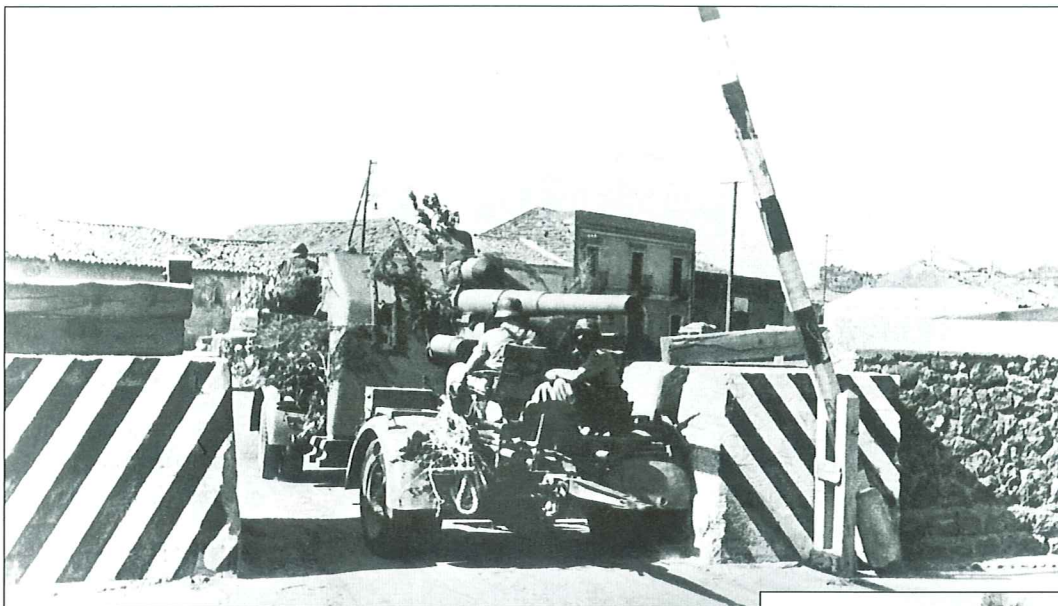
An 8.8cm FlaK 36 with a FlaK 18 barrel being towed into a town in Italy in 1943. Note the different type of gunshield that has been fitted. At the beginning of the war, most of the "88"s were organized into independent Luftwaffe anti-aircraft units, but since 1941, the number of these guns organized into the Panzer divisions had steadily increased.
